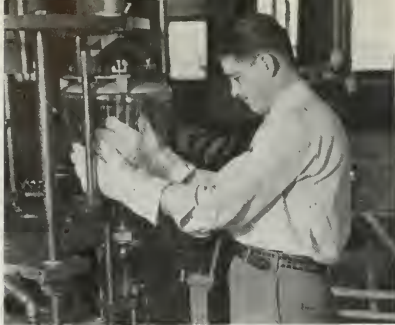
ABOVE: A 12-INCH KINESCOPE GOES THROUGH A FINAL STEP IN ASSEMBLY AT RCA VICTOR PLANT. RIGHT: A BATTERY OF NBC TELEVISION CAMERAS FOCUS ON THE ACTIVITIES AT AN OUTDOOR SPECIAL EVENT.
